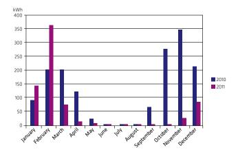
House B: Heated through a combination of an air-source heat pump and ECO forced-air heaters. Winter 2011 included a period when people were not present in the house and the floor heating, for example, was minimised. This is reflected as a peak in the energy consumption of the ECO heaters.
