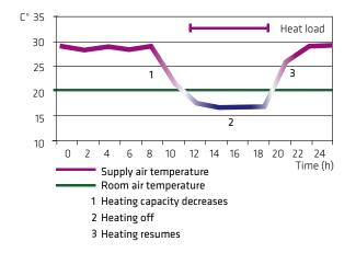
The graph shows the drop in supply air temperature with an additional heat load in the room, such as heat from the sun, fireplace or people. Supply air temperature drops below room temperature to compensate for the additional heat load and maintain a constant room temperature.
