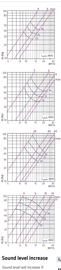
cover distance is below 3xØd: - after bend +4 dB (A) - after T joint +8 dB (A)
