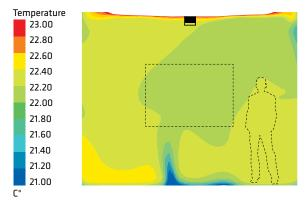
The temperature distribution within the entire room space is extremely even in passive houses and its rooms heated with ECO forced-air heaters. The cooler area at the front of the graph was caused by cooler air through the window.
